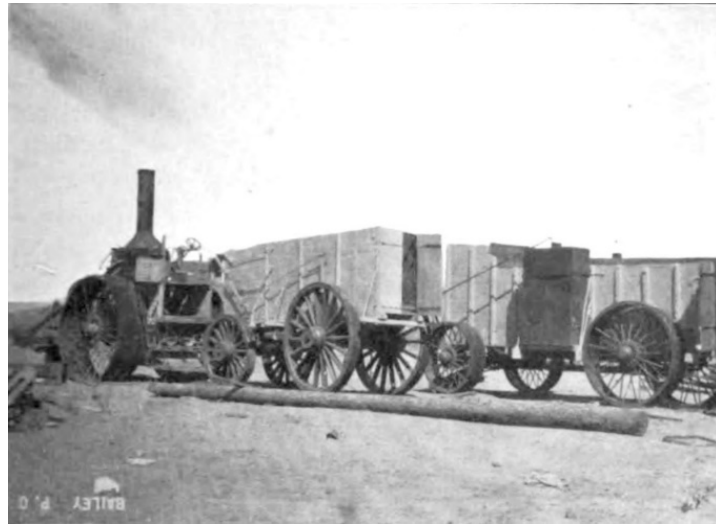
Osborne's "self-propelling wagon-train" sitting at Danby. Photo Bailey (1902, p. 129).
